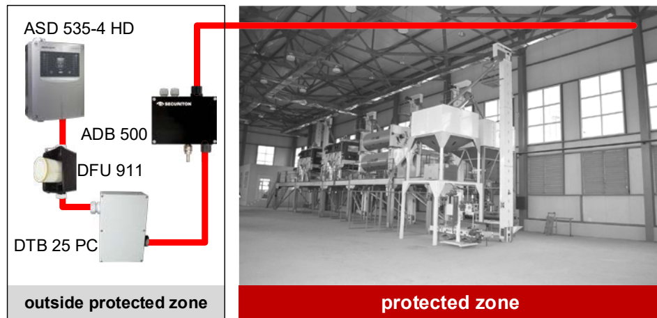
(a) High IP rating enclosure and very dusty environment (e.g. grain storage)
